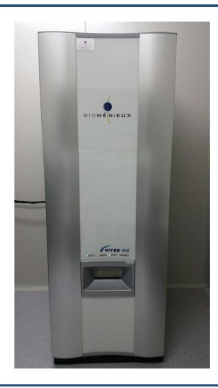
VITEK® MS is an automated mass spectrometry microbial identification system that uses Matrix Assisted Laser Desorption Ionization Time-of-Flight (MALDI-TOF) technology.
