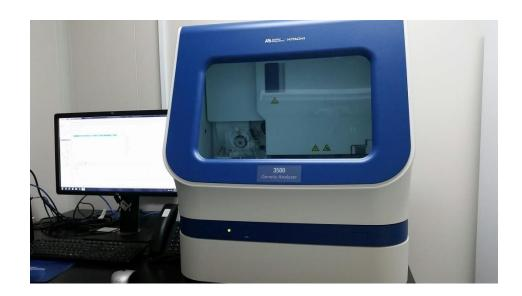
After sequencing the rRNA gene, the MicroSEQ® system automatically compares the results to validated sequences in the MicroSEQ® microbial libraries. The results are ranked according to genetic distance of the reference sequences to the sample and displayed on the system monitor along with a phylogenetic tree.
