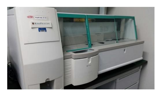
The DuPont™ RiboPrinter® System automates restriction fragment length polymorphism (RFLP) analysis and targets the rRNA-coding region of the bacterial genome. Only suitable for bacterial ID's.
