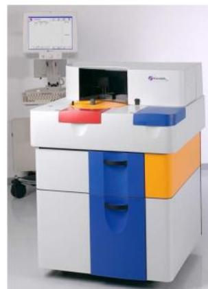
Nutrient analysis forms a large part of our business and we achieve this through the use of Flow Injection and Discrete Autoanalysers. These instruments perform nitrogen and phosphorus analyses and are also used to determine ammonia, cyanide, and hexavalent chromium. They take slow, manual colorimetric tests and automate them to speeds that are quite amazing.
