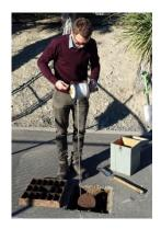
Eurofins-ELS is IANZ accredited for sampling the soil in the swale and basin and the process requires the removal of the grass and the collection of the soil layer beneath at the depth required by the local authority Resource Consent. It is usual for two to three samples to be collected from around the swale/basin and composited into a single sample for analysis.
