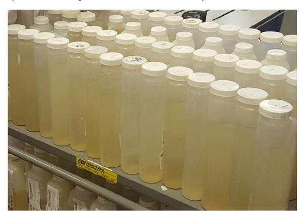
Laboratory analysis can be used to find sewer breaks and illegal sewer connections. Elevated microbiological counts can indicate a source of sewage, as can some chemical analyses.
