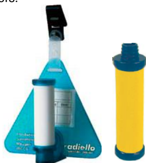
Figure 1: radiello® RAD130 arranged in sampling plate and yellow low-uptake diffusive body
