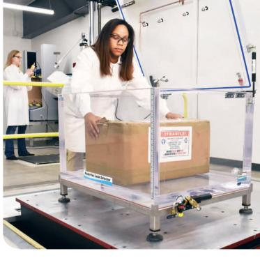
Distribution Testing: No matter how or where your product is shipped, Eurofins Medical Device Testing's state-of-the-art distribution testing equipment can simulate the stresses of shipping on products. Standard ASTM and ISTA distribution cycles, as well as custom programmes, can be performed that simulate stacking, manual handling, and vibrations associated with various forms of transport, as well as pressure changes that can be seen during air or mountainous product transportation.
