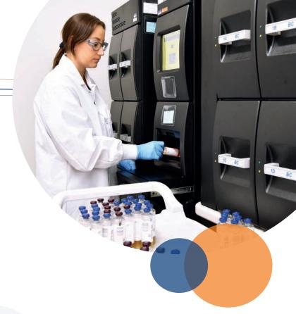
If microorganisms are present in the test sample, CO2 is produced as the microorganisms metabolize the substrate found in the culture medium. When growth of the microorganism produces CO2, the color of the sensor located in the bottom of each culture bottle changes from dark to light. A light emitting diode (LED) projects light onto the sensor, which is then reflected and measured by a photodetector.
