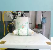
In 1991, Eurofins launched SCAN 1, a first-of-its-kind testing device for diapers (nappies). This exciting dynamic "model baby" offered a valuable validation tool and the first alternative to costly and hard to implement consumer panels. Not only did it allow Eurofins to provide very real technical feedback, but also to simulate realistic user conditions. Since its birth, the device has evolved into a third iteration - SCAN 3.
