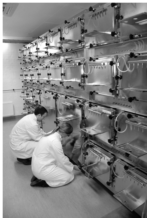
Figure 3. VOC emissions are tested in ventilated stainless steel climate chambers.
