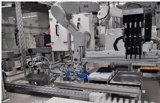
Example Contaminants Testing Automation System
