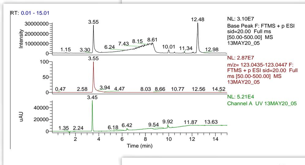
**FIGURE 6.** Example chromatograms of tropolone (1 mg/mL) exposed for 30 min, diluted to 10 ppm in water. **Top:** base peak chromatogram; **Middle:** extracted ion chromatogram m/z 123; **Bottom:** UV 254 nm.
