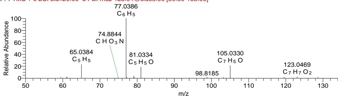
**FIGURE 15.** MS/MS spectrum of peak 4 MS2 scan of m/z 123.
