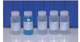
\* The sampler will receive the Trip Blank (TB) filled with water and preservative. It is colored in the picture to indicate the bottle is filled (not empty) for picture purposes only. \*\*The sampler will also receive an empty bottle labeled @537 FB (Field Blank) and 3 sets of preserved bottles.
