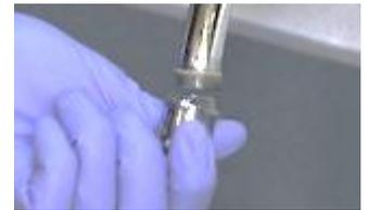
6. Open the tap and let the water of the sample source run at fast flow for approximately 5 minutes.
