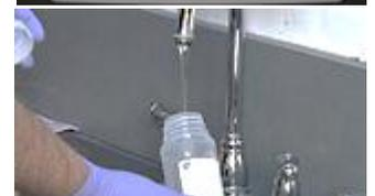
9. Fill sample bottle up to **bottom of neck**, taking care not to flush out preservatives and making sure the mouth of the bottle does not come in contact with anything other than sample water.
