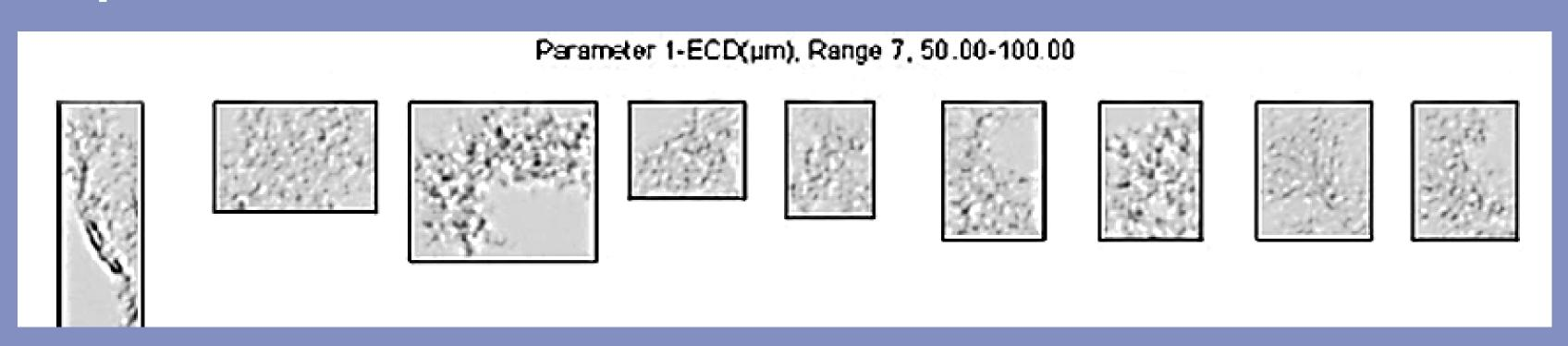
The MFI has been proven to have the ability to screen for the presence of translucent particles (see image above) that may have been missed by light obscuration methods, due to light passing directly through the particles.
