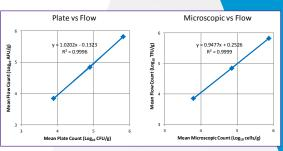
Figure 5. An example of comparable results produced by flow cytometry and standard plate counting (left) and flow cytometry and direct microscopic counting (right).
