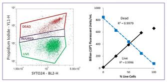
Figure 3. Example of specificity testing showing differentiated live and dead cell populations. Left: flow cytometry scatter plot showing different populations. Right: plot of resulting test data.
