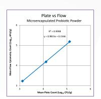
Figure 6. Comparable enumeration results were produced for microencapsulated probiotic powder by flow cytometry and standard plate counting.
