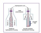
Figure 1. Rapid, improved alignment with acoustic focusing.
