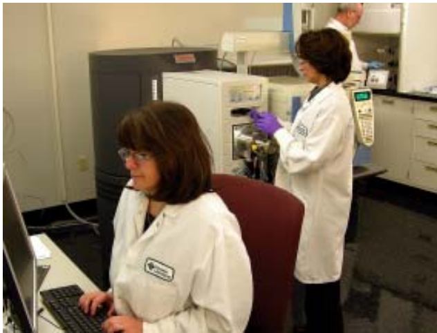
Analysts perform dioxin testing in Lancaster Labs' newest lab, which features a Thermo Scientific DFS high resolution gas chromatograph/high resolution mass spectrometer.
