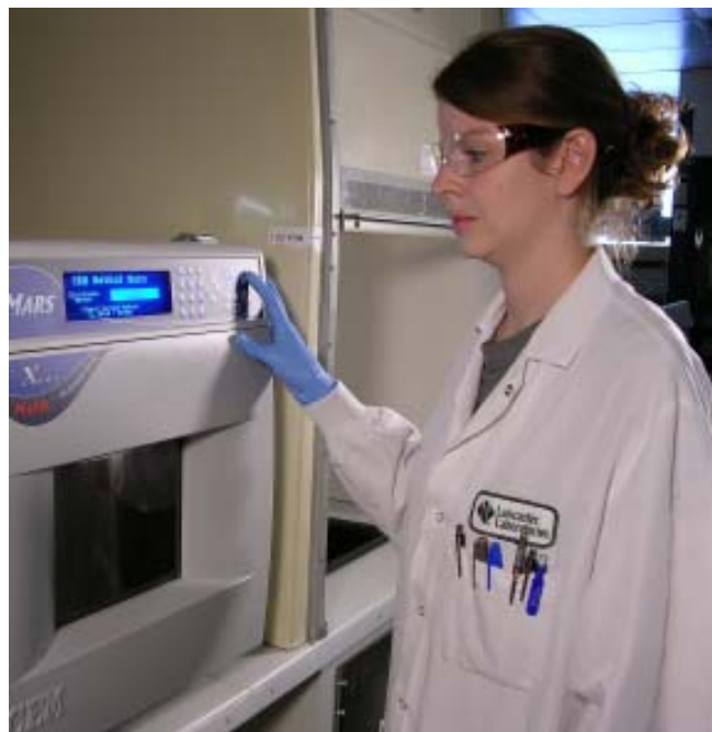
Kerrie Freeburn, chemist in the Organic Extractions Department, performs microwave extraction for semivolatile organic compounds.
