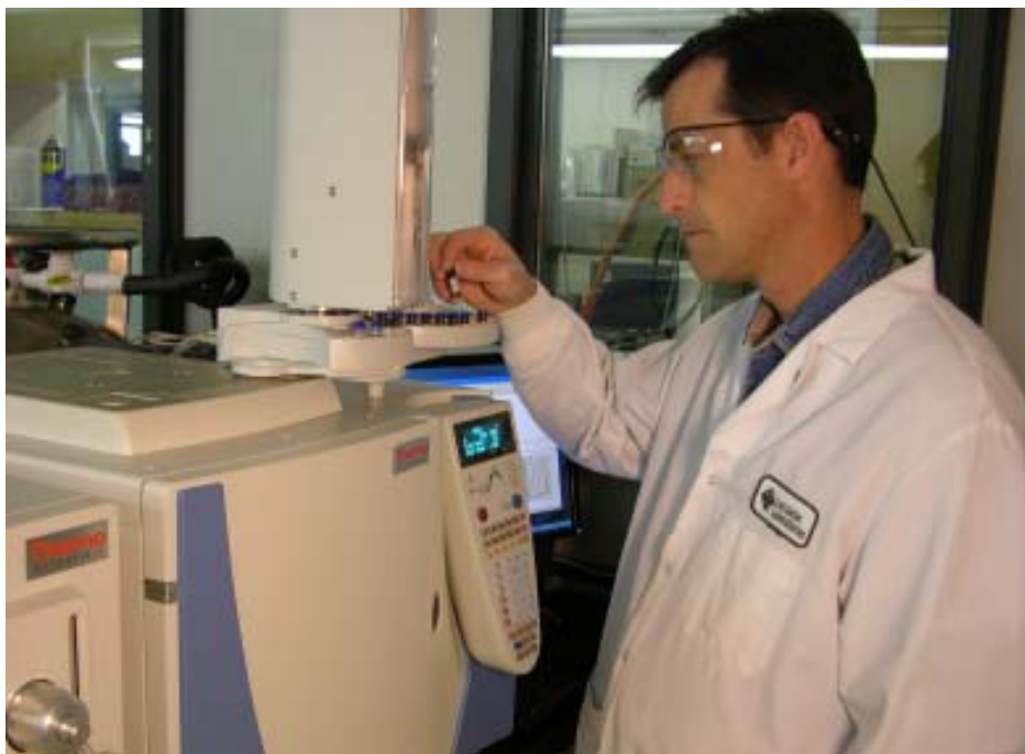
Tim Trees, principal chemist in the GC/MS Semivolatiles Department, analyzes water samples on a new Thermo Scientific DSQ II GC/MS instrument.
