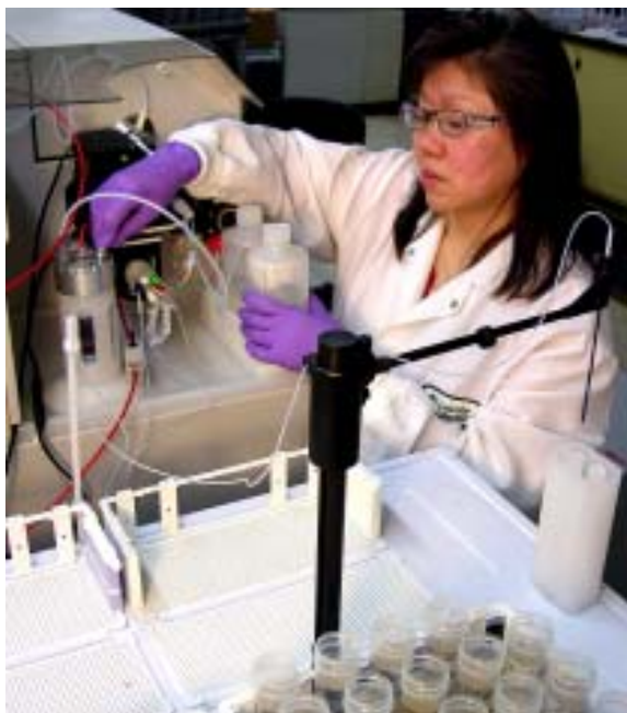
Choon Y. Tian, analyst, avoids arsenic false positives on soil samples by using ICP/MS with CRC and HMI.
