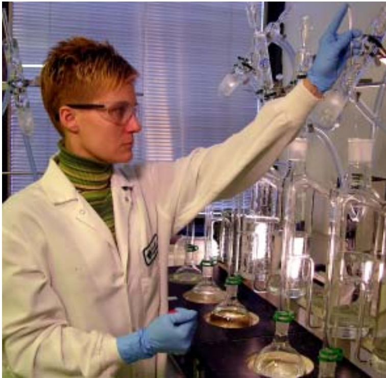
Heidi Ortenzi, senior chemist, spikes a liquid/liquid extractor on water samples for the detection of NDMA at low PPT levels.
