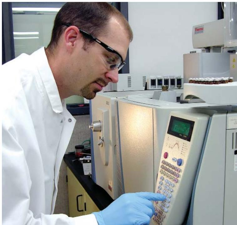
**Chad Moline, Senior Chemist, analyzes water samples for N-Nitrosodimethylamine using a Thermo Scientific Trace Ultra GC and DSQ II Mass Spectrometer.**
