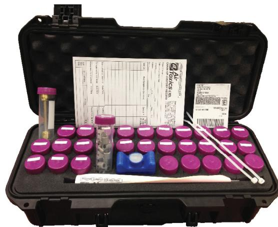
Eurofins Air Toxics has developed a media inventory and management program to meet method requirements and provide the field technicians with convenient, simple-to-use sampling kits in order to streamline sampling and minimize errors. The sampling kit consists of a rugged shipping case with custom foam inserts to organize the individual sorbent tubes packed in storage vials and other sampling equipment such as extra diffusive caps and disposable nitrile gloves.
