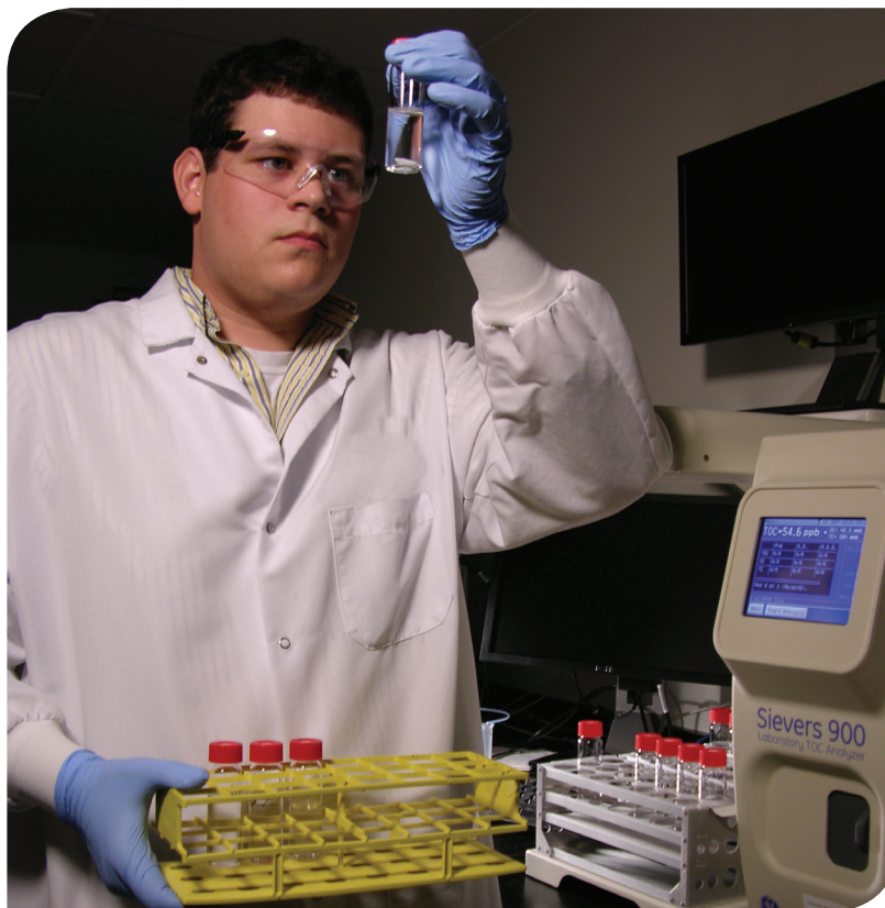
Chemist Anthony Langione inspects collected swab samples before loading them onto the TOC analyzer.
