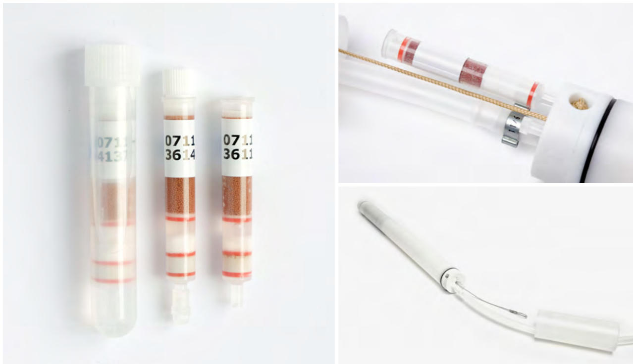
Figure 1. Picture left: SorbiCell VOC. From left to right: unexposed, as purchased in transportation tube; exposed, fitted with protection caps; exposed Sorbicells with about 50% salt depletion. Pictures on the right: GWS-40 mounting units for installation of SorbiCells in groundwater wells.
