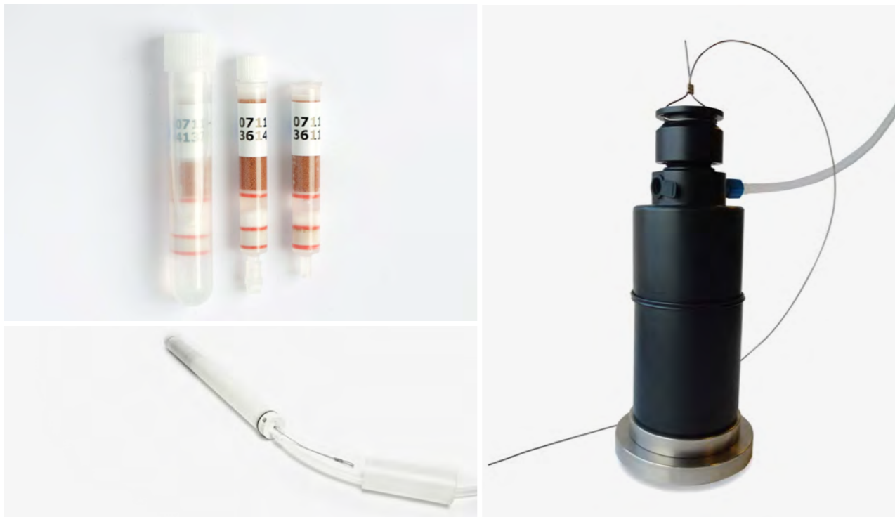
Figure 1. Pictures of SorbiCell VOC. Left picture, from left to right: unexposed, as purchased in transportation tube and pre-wetted in de-mineralized water; exposed, fitted with protection caps to prevent drying; exposed Sorbicells with about 50% salt depletion. Picture right shows field mounting units WW-50 (TOP) and GWS-40 (BOTTOM)
