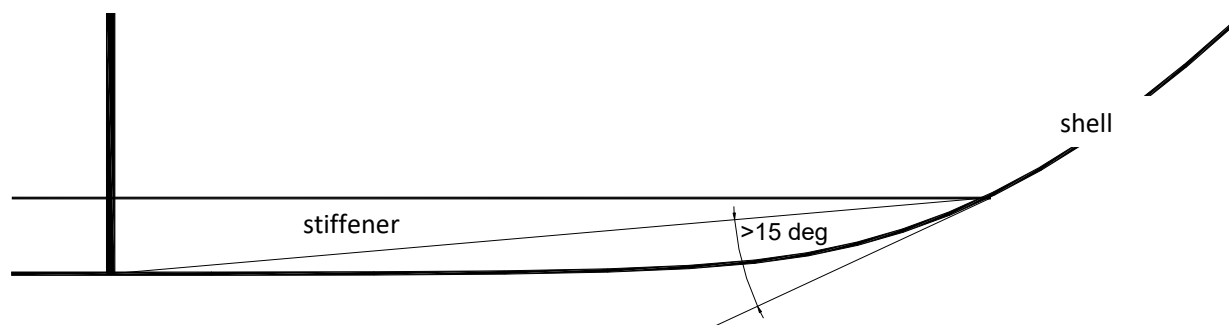
Figure 8.2. The stiffener runs out against the hull shell.
