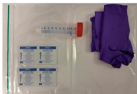
Fig 1. Eurofins surface wiping kit containing four isopropanol wipes (one extra), one 50 ml tube and a pair of nitrile gloves
