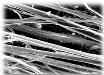
SEM adhesive sample chrysotile (white asbestos)
