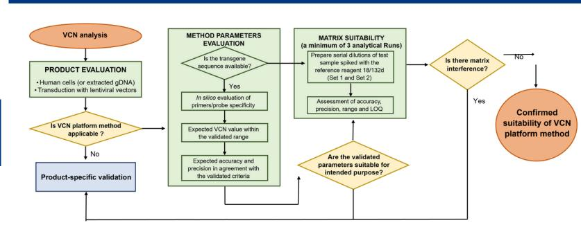
Flowchart describing the analytical steps for the method parameter and matrix suitability evaluation.
