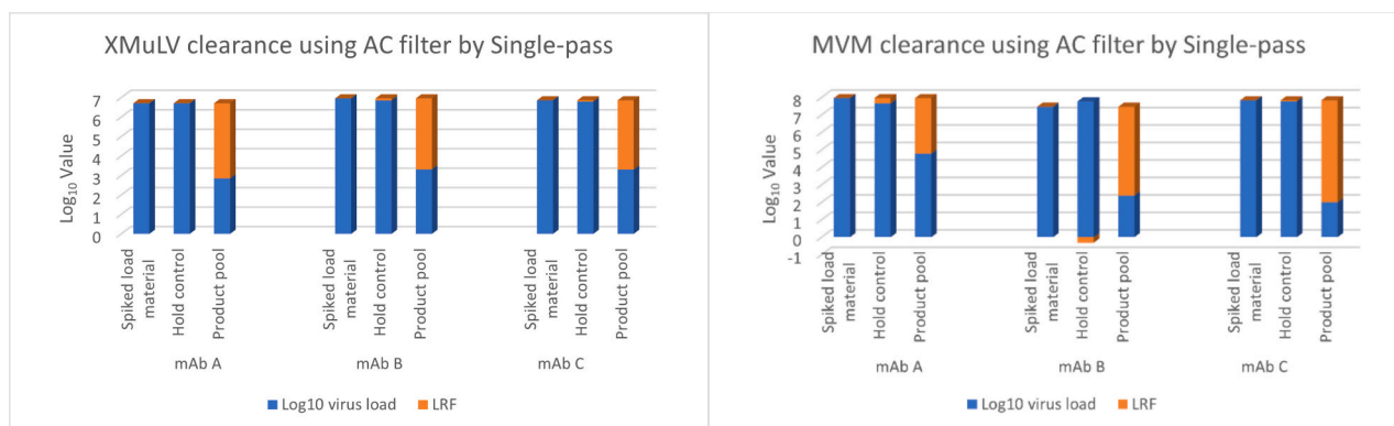
Fig. 3. Viral clearance achieved through a column-free single-pass filtration approach using activated carbon (AC) filters. The histograms report the LRVs for MVM and X-MuLV viruses when spiked into three different monoclonal antibody preparations (mAb1, mAb2, mAb3). The comparison includes: i. Hold Control – untreated spiked samples incubated under test conditions to assess virus stability; ii. Spiked Load Material – virus-spiked input prior to AC filtration; iii. Product Pool – filtrate collected after AC processing (Kikuchi et al., 2022).
